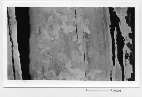
Plate 14. Strip SF1824, ferrite surviving between the corroded edges. Nital etch.
