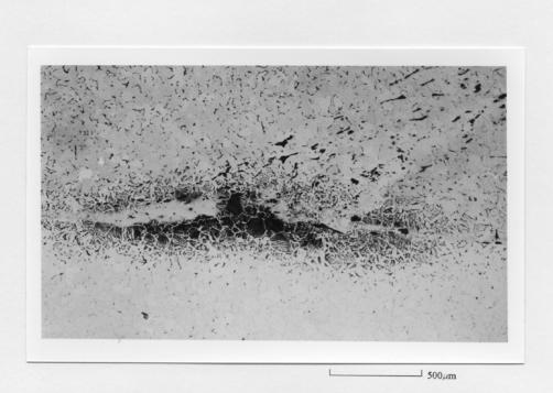
Plate 5. Split bar SF1595 flat end. Part of weld line (centre) with slag inclusions within, surrounded by pearlite (dark). Nital etch.
