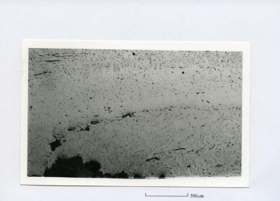
Plate 11. Plate SF1660. Banded structure: mottled ferrite (centre) outlined by slag inclusions, between two low-carbon bands of pearlite (top and lower). Nital etch.
