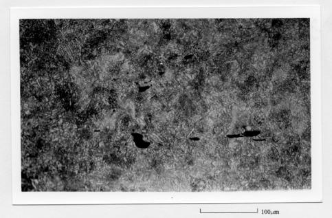
Plate 4. Bar SF1594, showing high-carbon steel of eutectoid composition at the bar end. Pearlite (dark), glassy inclusions (black). Nital etch.
