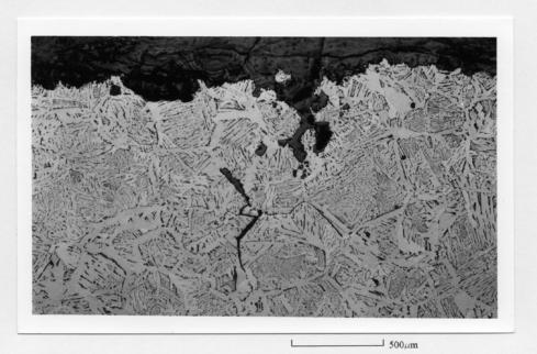
Plate 9. Notched bar SF1627, edge of specimen showing ferrite and pearlite with Widmanstätten appearance. Carbon concentration is c. 0.3%. Nital etch.
