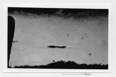
Plate 10. Folded strip SF1633, showing ferrite predominating (light) and a narrow zone of pearlite at one edge (upper, grey zone).
