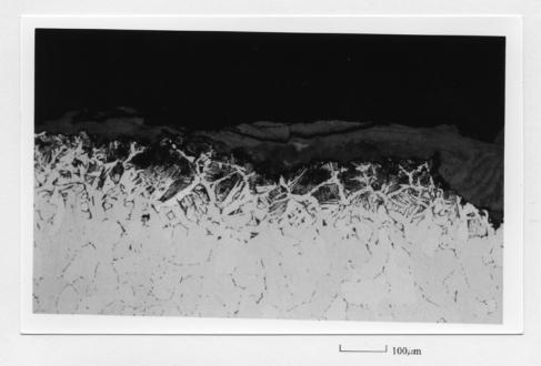
Plate 6. Split bar SF1595 flat end, showing carbon concentration at the metal surface (top), visible as a pearlite (centre) adjacent to ferrite (lower). Nital etch
