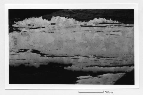
Plate 8. Folded strip SF1608, showing ferrite (light) and slag stringers and corrosion running through the specimen. Nital etch
