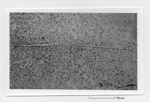
Plate 3. Tapered bar SF1590. Transverse specimen from mid length showing weld line plus a lower concentration of pearlite. Nital etch.
