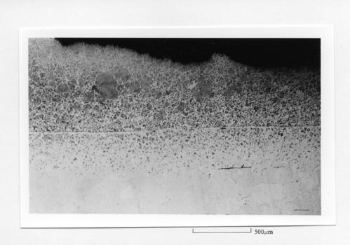
Plate 1. Tapered bar SF1590. Specimen from wide end showing ferrite grains (pale, lower) and pearlite (dark) at the metal surface (black, upper). Across the centre (left to right) is a light-etching weld line. Nital etch.
