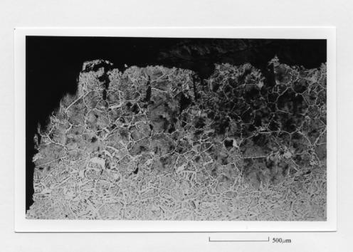
Plate 7. Split bar SF1595 transverse section, showing a broad zone of pearlite at one surface. Nital etch.
